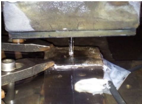
Fig. 3. Coating of strain gauge.
