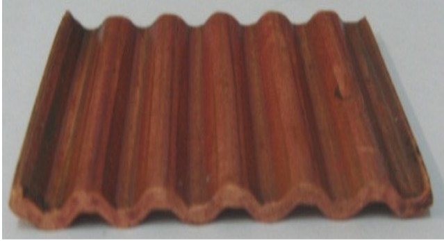
Fig. 5. Copper sample after pressing the 5 times.
